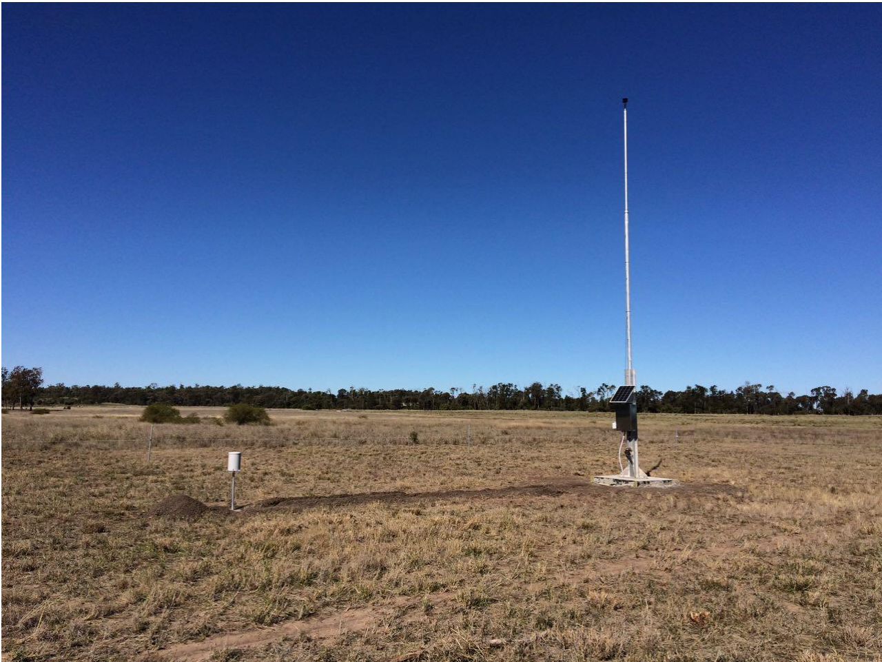
Figure 7-6 Indicative Air Quality and Atmospheric Monitoring Station (top of mast is 10 m above ground level)
